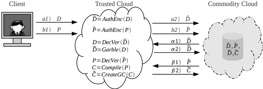
**Fig. 3.** *Setup Phase:*  $a, b$ ) Client registers data  $D$  and program  $P$  to be stored securely in the *Commodity Cloud*.  $\alpha$ ) Updates of  $D$  require re-generation of garbled data  $\tilde{D}$ .  $\beta$ ) Updates of  $P$  require re-generation of garbled circuits  $\tilde{C}$ .
